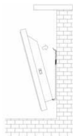
Figure 7. Attaching upper hook of the wall mounting brackets to the convecter
