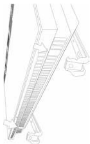
Figure 6. Placing the convecter to the lower part of the wall mounting
